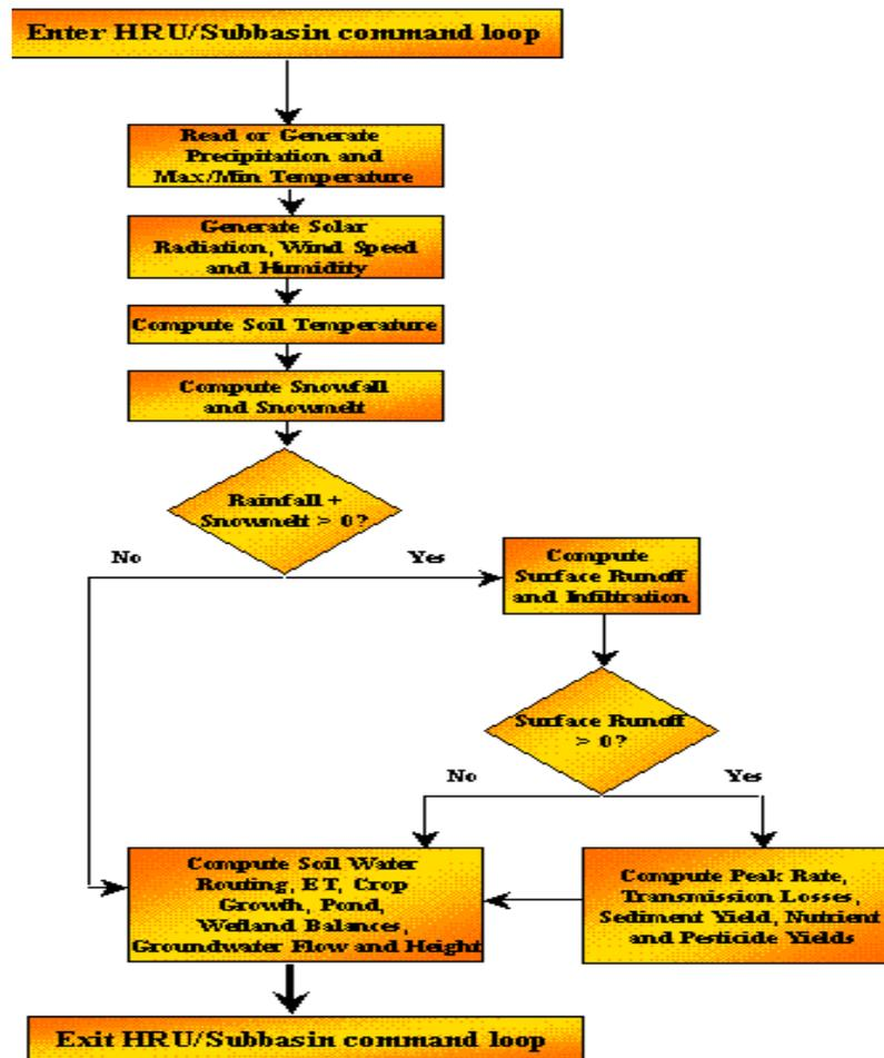
Figure 2.4: HRU/Sub basin command loop
