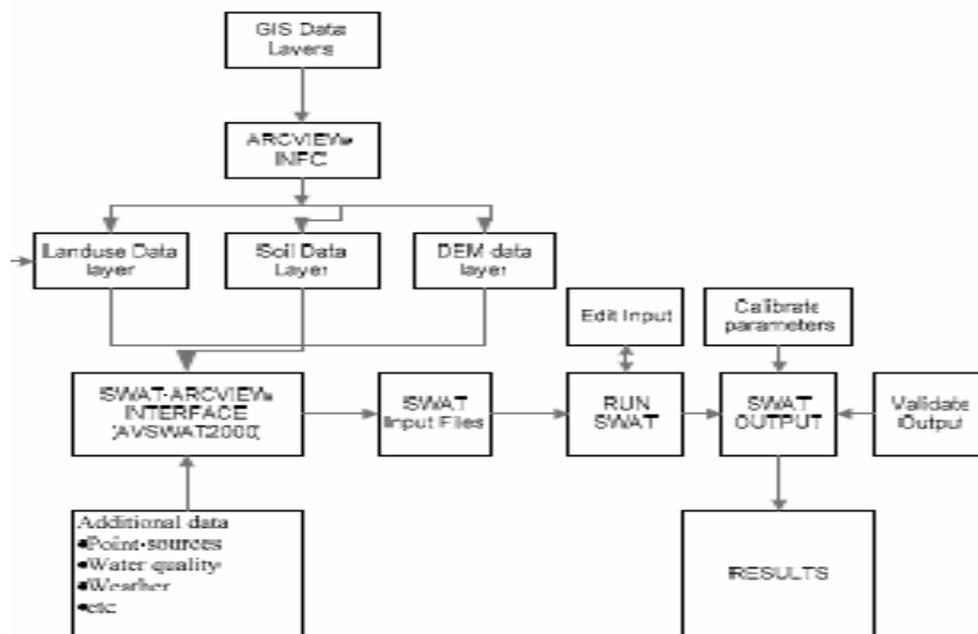
Figure 4.1 The general layout of Simulation diagram of SWAT model
