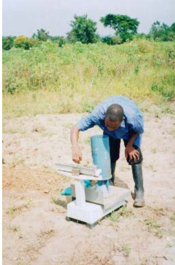
Weight measurements for in-situ density tests
