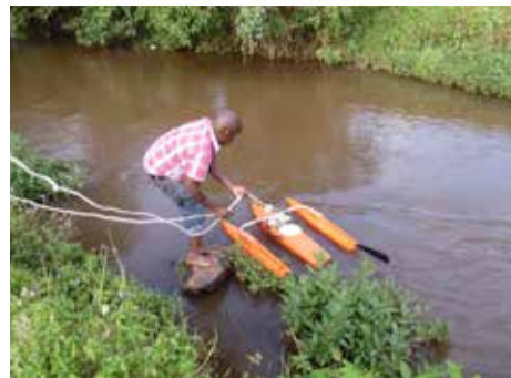
ADCP being lowered into the the stream
