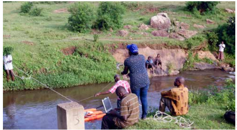
Taking ADCP readings
