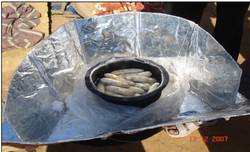
Plate (1): Solar Energy Cook stove in Ntarama Sector.
