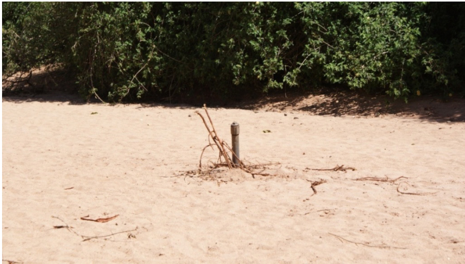
Figure 4.5 Piezometer within sand storage dam (source Alemu Seifu, 2011)
