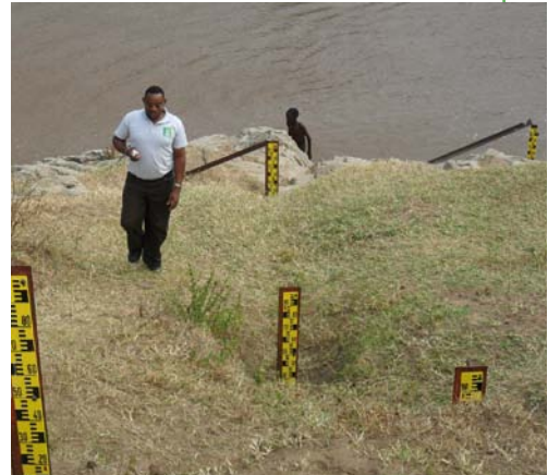
A gauging station recently installed as part of the NBI Mara River Basin Management Project.
