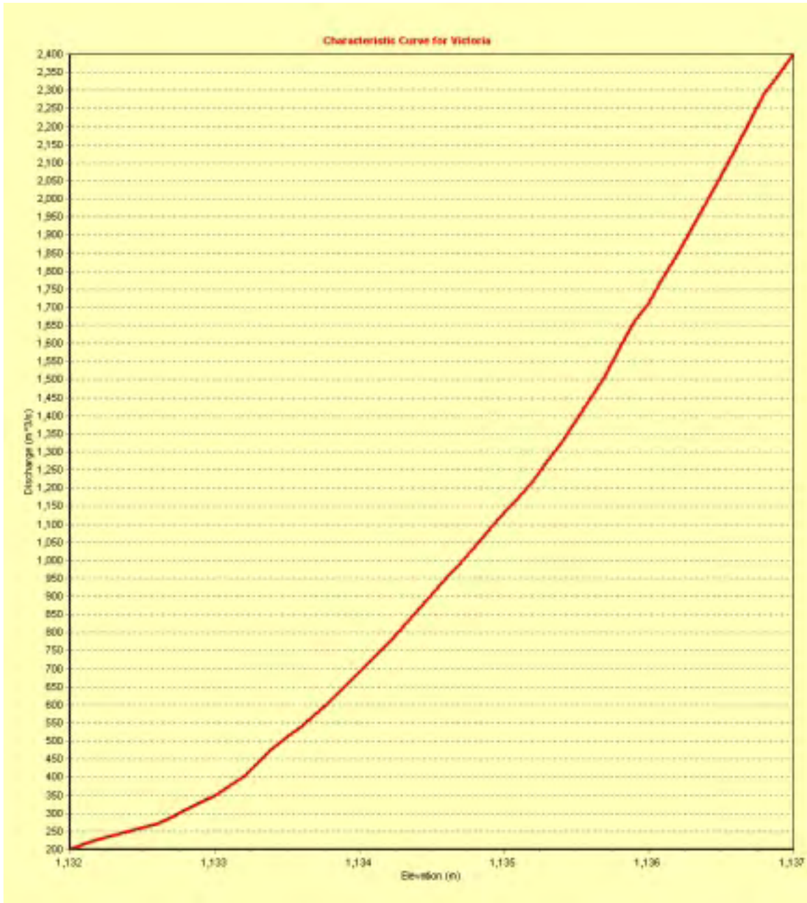
Figure 5.1: Natural Outflow Curve for Lake Victoria
