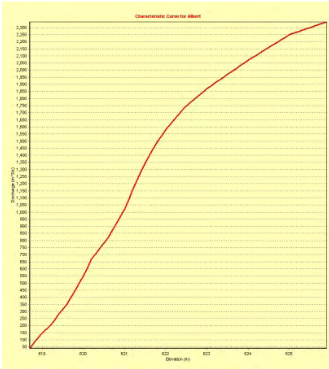
Figure 5.3: Natural Outflow Curve for Lake Albert
