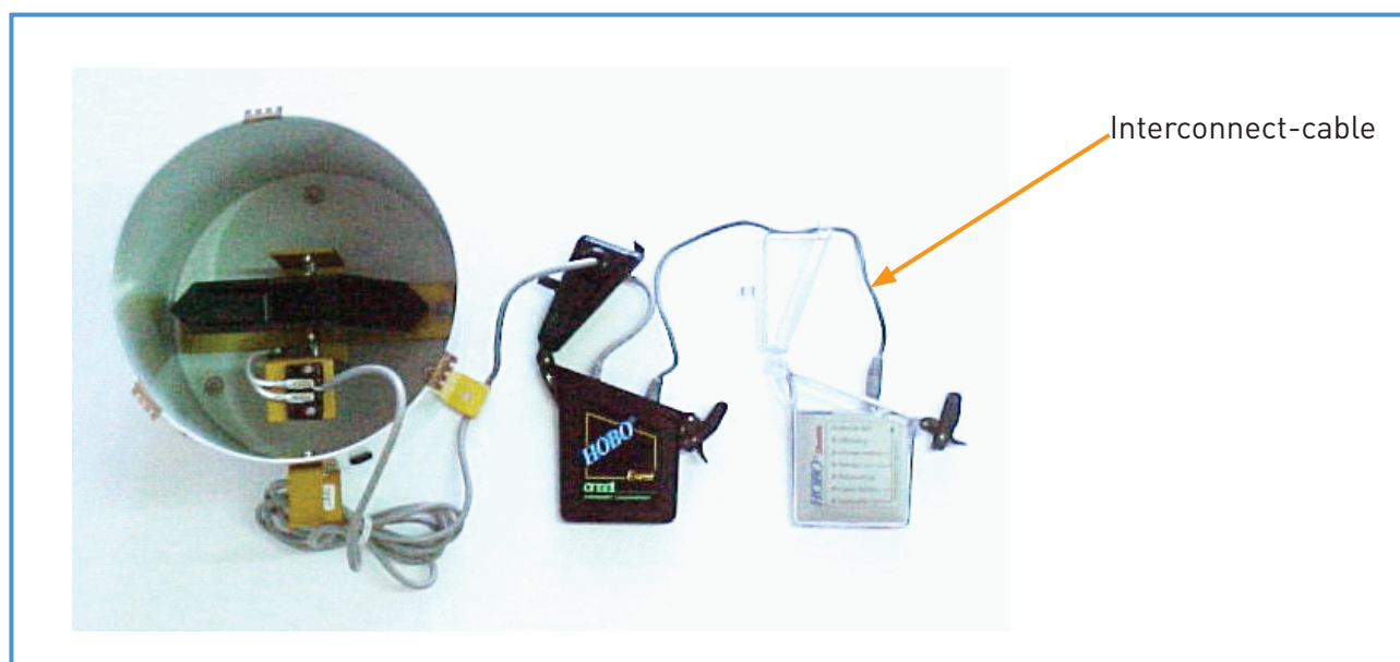
Figure 11: Connecting the HOBO Shuttle to the HOBO Event Logger
