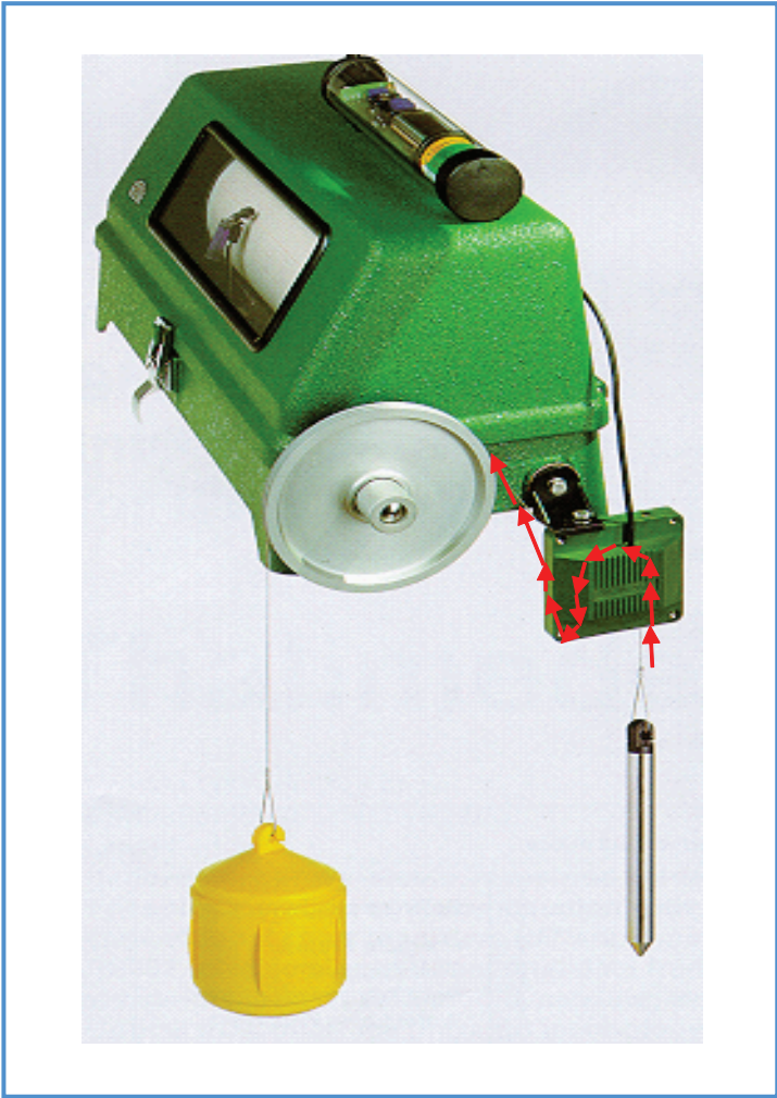
Figure 7: Attachment of Thalimedes to OTT Horizontal water level “Type X”
