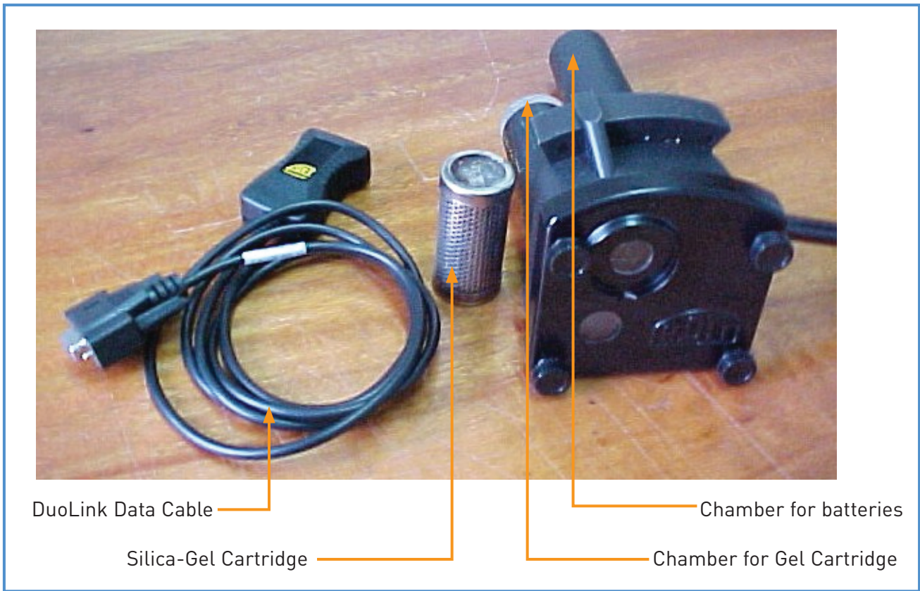
Figure 2: Standard logistics unit with data readout cable
