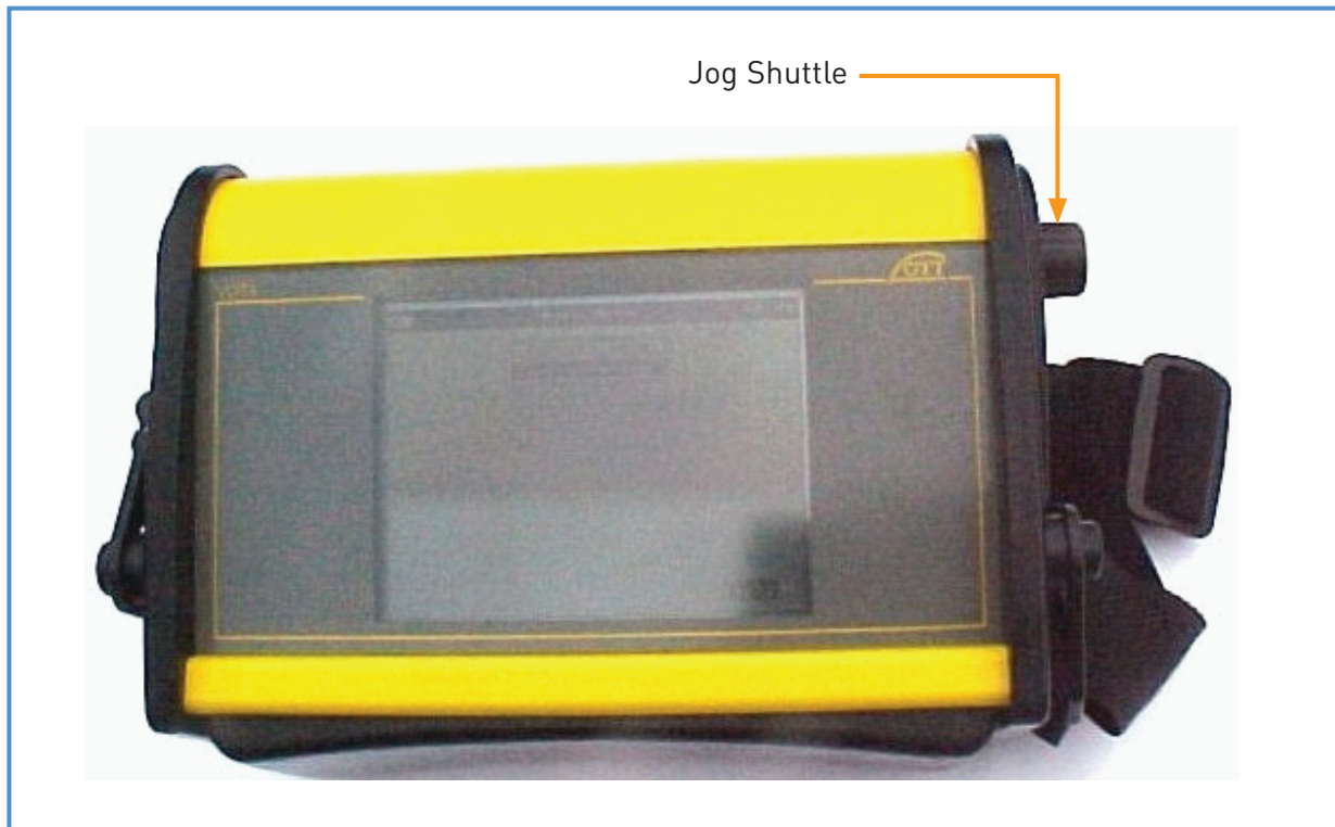
Figure 3: OTT VOTA programming / retrieval unit
