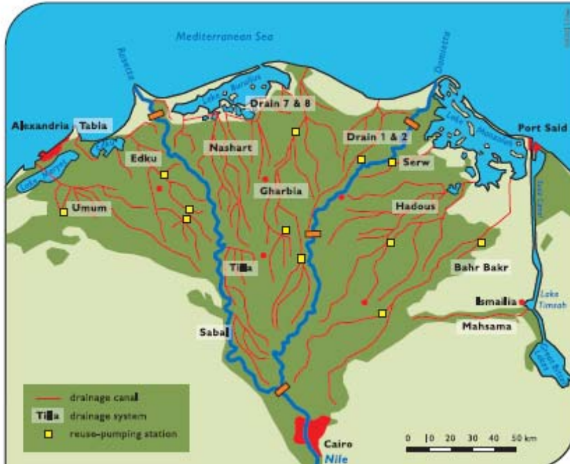
Figure 2-6 Main drainage canals in the Delta
