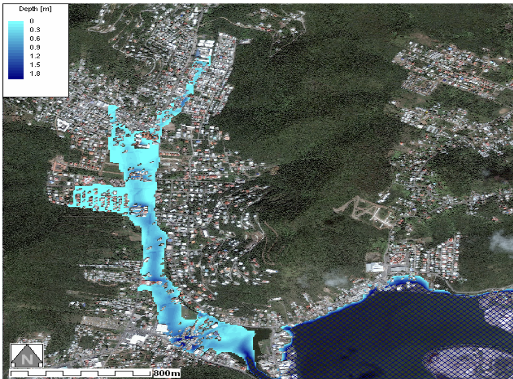
Figure 22: Water depth-Smooth with Road and Buildings_ DTM10_M30 Aerial Photo
