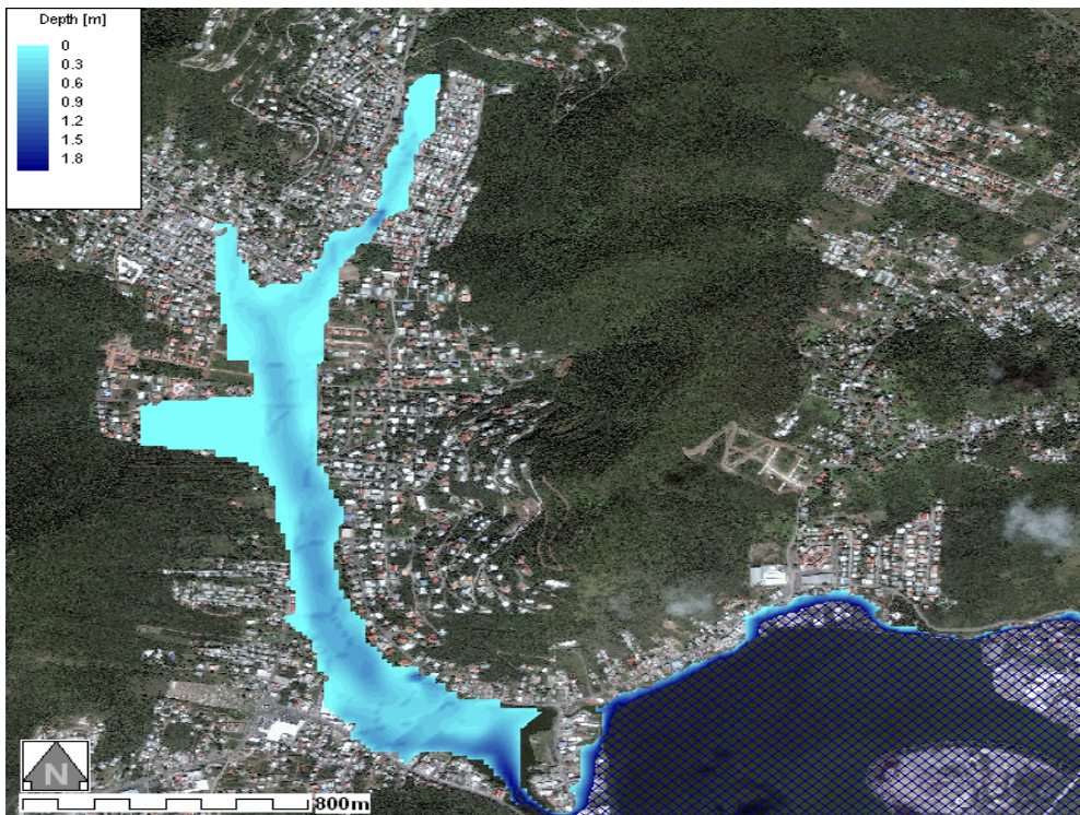
Figure 11: Water depth-Smooth with Roads DTM15_M20 Aerial Photo
