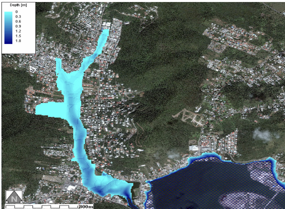
Figure 10: Water depth-Smooth with Roads DTM10_M20 Aerial Photo
