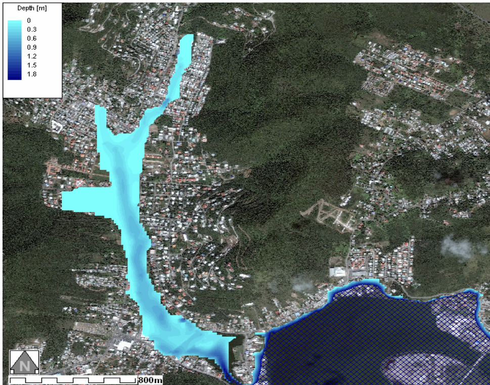
Figure 7: Water depth-Smooth DTM15_M30 Aerial Photo
