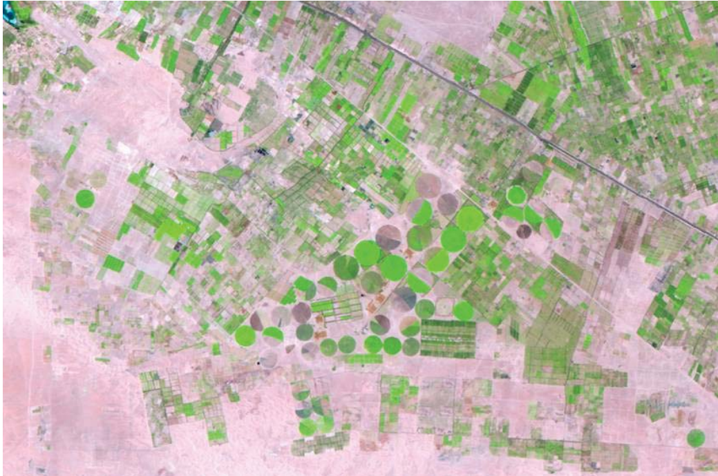
Detailed Landsat Thematic Mapper picture of the Dina farm along the Desert Road. This commercial farm was visited on September 16 th . The circular features are center pivot systems present on the farm with sprinkling irrigation. The rectangular structures show orchards with drip systems. The white line from southeast to northwest is the Desert road.
